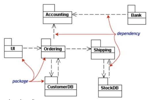
Fig. 8: an example package diagram
