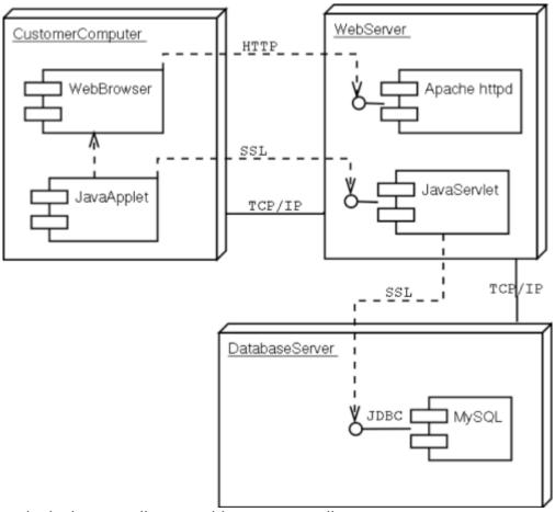
Fig. 6: an example deployment diagram with component diagrams
