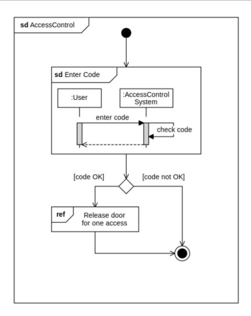
Fig. 14: an example interaction overview diagram
