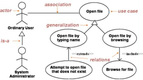
Fig. 12: an example use case diagram
