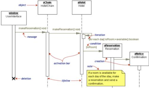
Fig. 15: an example sequence diagram
