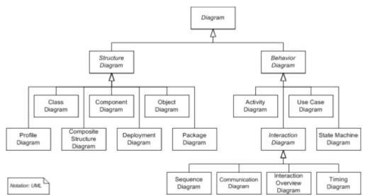
Fig. 1: Diagrams of UML 2.2
