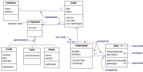
Fig. 2: An example class diagram
