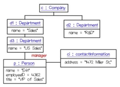
Fig. 7: an example object diagram
